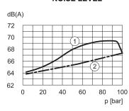
Approximate maximum values of noise level to minimum and maximum flow rate measured with the sound-level meter placed at one meter from pump coupling with flexible coupling.
