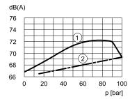
Approximate maximum values of noise level to minimum and maximum flow rate measured with the sound-level meter placed at one meter from pump coupling with flexible coupling.
