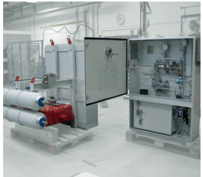
Hydraulic power station to control valve actuators used to isolating the oil pipeline
