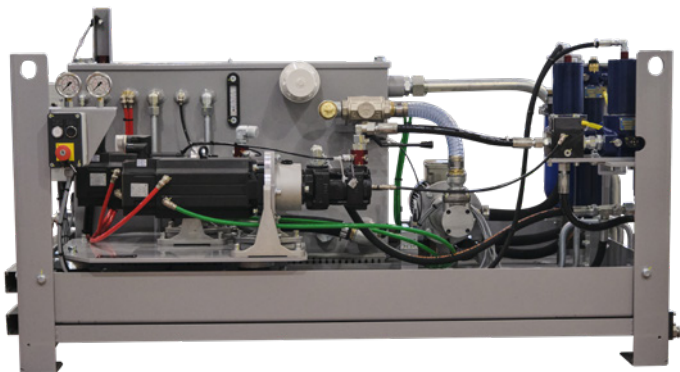
Power unit for punching machine with servo pump
