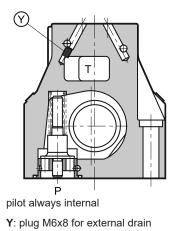
**NOTE**: the backpressure valve can't be used as direct check valve because it doesn't assure the seal.
