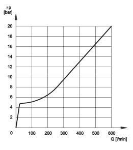
The curve refers to the pressure drop (body part only) with backpressure valve energized to which the pressure drop of the reference spool must be added. (see paragraph 5)
