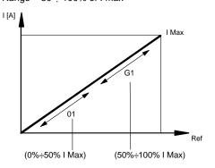
o1: "OFFSET1" current, expressed in milliampere. It sets the offset current to the solenoid, when the reference
