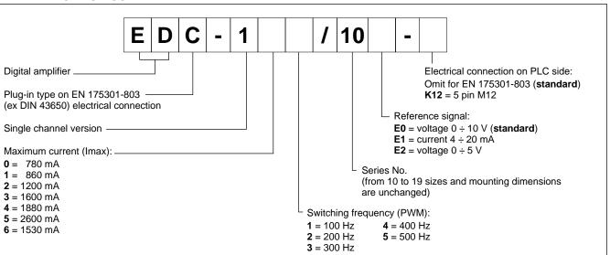
The EDC-1 is a digital amplifier for open-loop control of proportional valves with DIN-type coils, to be plugged directly onto the valve's electrical connection.
